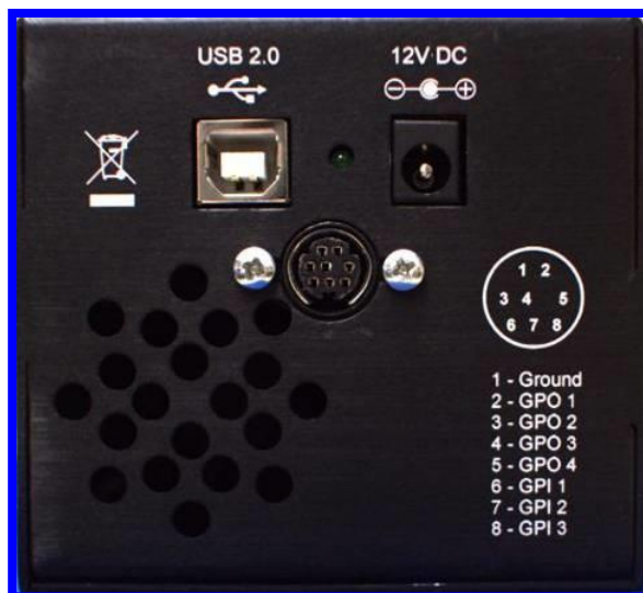
Figure 28: Large Format Camera External Header Location and Pin Numbering
